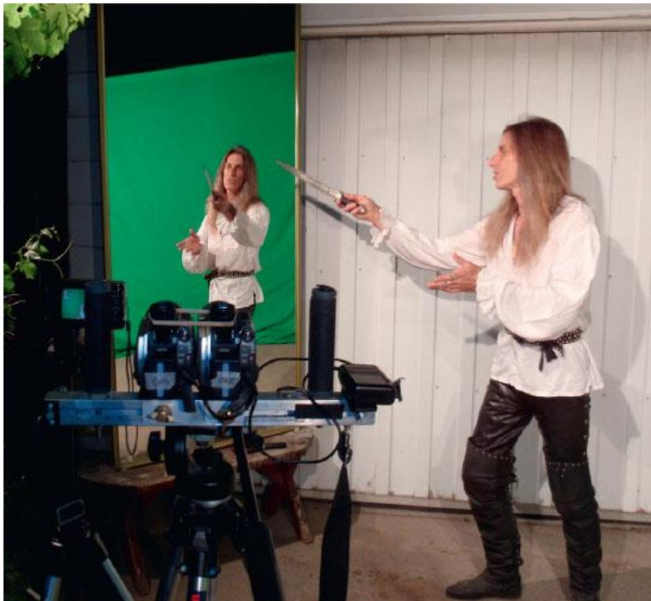
**Figure 23.28** A green-screen setup with side-by-side cameras in the foreground shooting the actor in a mirror with a green-screen background.
