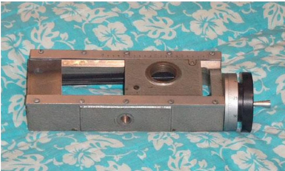
**Figure 23.16** A custom "twin bar" with variable interaxial built by Razutis for shooting 3D with a variety of digital cameras side by side.
