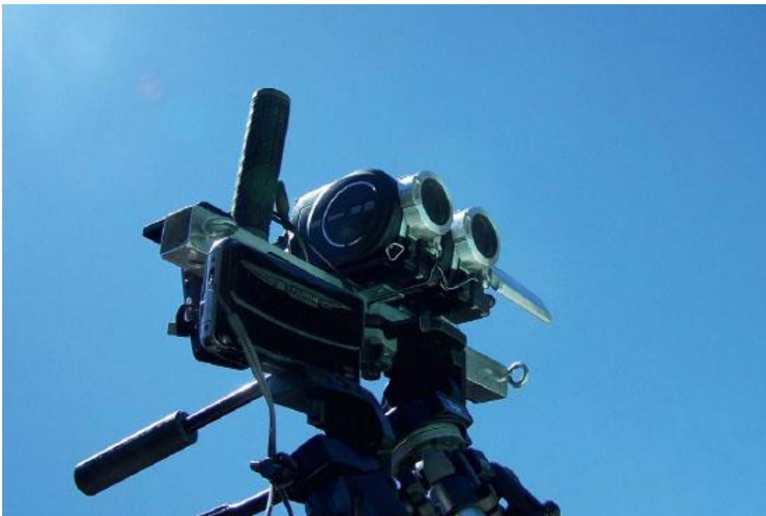
**Figure 23.24** *On a single tripod, Razutis has paired two HD cameras side by side with a Fujitsu 3D camera.*
